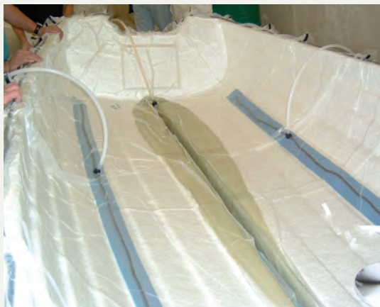
Fig. 3 Scott Bader offre la serie di resine Crystic per stampi chiusi con infusione a vuoto, RTM leggero e RTM Scott Bader also offers a range of Crystic closed mould resins for vacuum infusion, RTM light and full RTM
